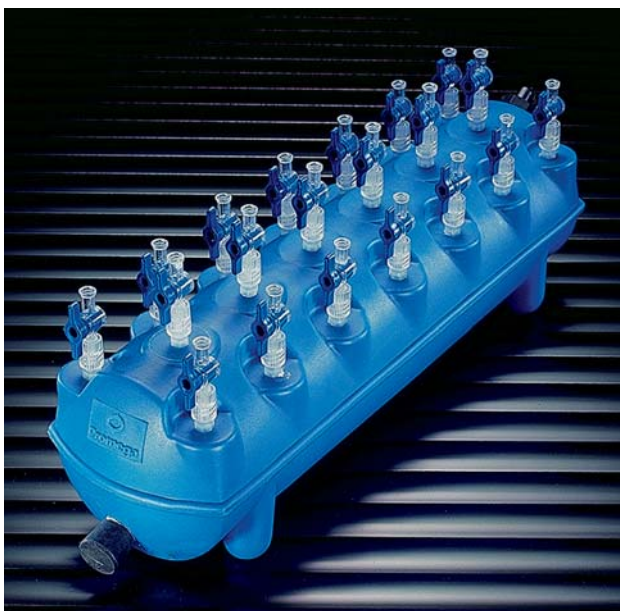
Figure 1. Vac-Man® Laboratory Vacuum Manifold.
